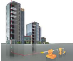
Pneumatic Waste Collection Systems
